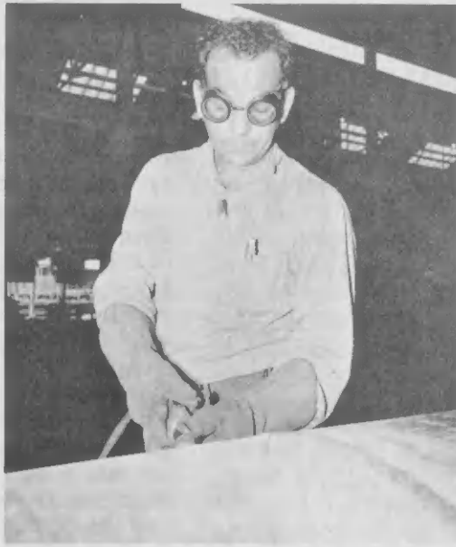
A chipper goggle protects the eyes of Martiliano Lopez while he performs a chipping job in the Welding Shop.
